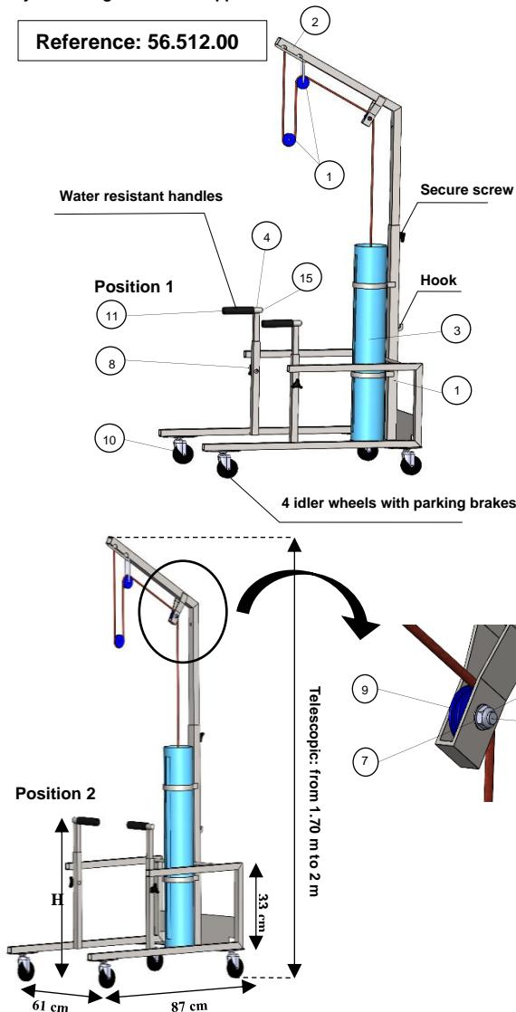
The device contains two pairs of handles of different sizes, to be selected based on the height of the patient. The low handles have two positions, shown above.
